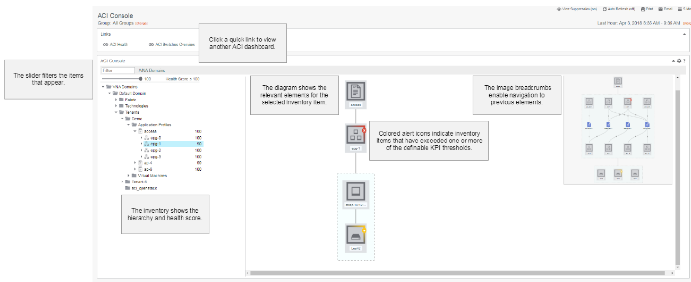
Figure 54: ACI Console Elements
